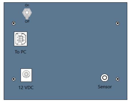
• Sensor Jack – Connects the meter to the remote sensor unit via a standard stereo audio cable. Accepts a standard 3.5mm stereo plug.
