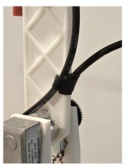
Pass the tie-wrap through the hole and wrap it snuggly around the cables to prevent them from: a) adding dead weight to the end of the elevation arm, and b) becoming snagged in the elevation position indicating gear train.
