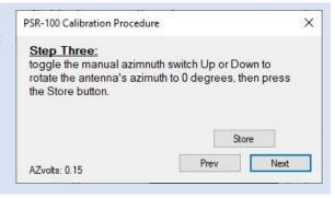
As instructed in the step three text, use the manual azimuth toggle switch to rotate the Elevation Motor Mounting Bracket so that it is at 0 degrees.
