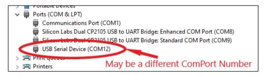
If there is more than one *USB Serial Device* entry, you can easily identify the one associated with the meter's USB controller by unplugging it and observing which entry disappears from the Device Manager listing.
