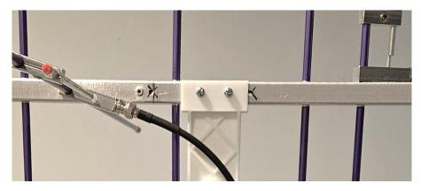
accommodate the **M4x0.7x30mm** mounting screws. One side of the mounting bracket is threaded, so no nuts are needed to secure the antenna to the bracket.
