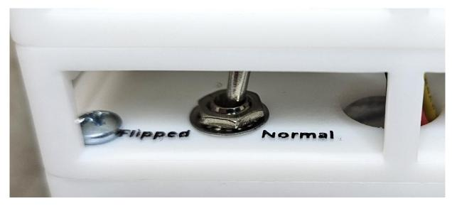
The operator should be able to activate the switch using their finger. If not, then a narrow probe such as a pen or pencil may be used.
