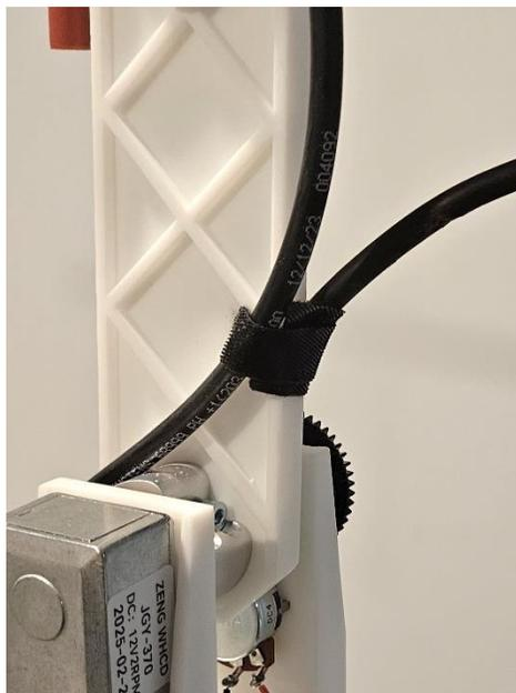
Pass the tie-wrap through the hole and wrap it snugly around the cables to prevent them from: a) adding dead weight to the end of the elevation arm, and b) becoming snagged in the elevation position indicating gear train.
