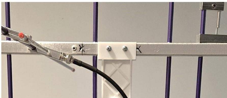
accommodate the **M4x0.7x30mm** mounting screws. One side of the mounting bracket is threaded, so no nuts are needed to secure the antenna to the bracket.
