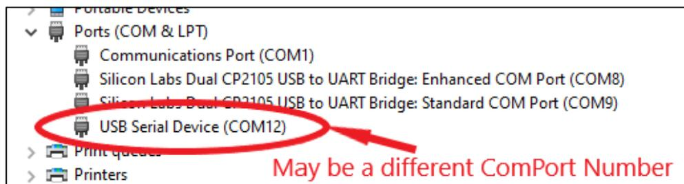
If there is more than one **USB Serial Device** entry, you can easily identify the one associated with the meter's USB controller by unplugging it and observing which entry disappears from the Device Manager listing.
